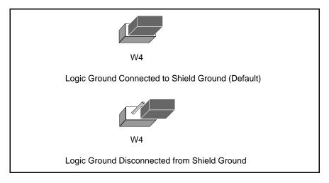
Figure 2-10. Ground Configuration Jumper Settings
